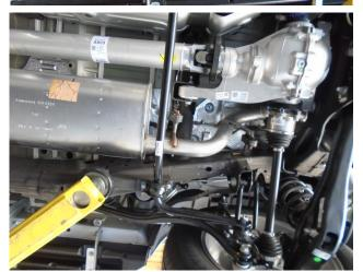
**Step 1.** To remove the OE exhaust system you will need to remove the spare tire, heat shield and sway bar. Unfasten the clamp attaching the OE inlet pipe assembly to the catalytic converter. Do not damage or discard the inlet pipe clamp or rubber insulators as they will be re-used to mount the new system. Working front to rear disengage the hangers from their rubber insulators and remove the exhaust from the vehicle.
