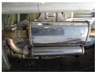
**Step 3.** Attach the Muffler Assembly to the Reasonator Assembly with a supplied 3.00" clamp. Engage the welded hanger to the rubber insulator.
