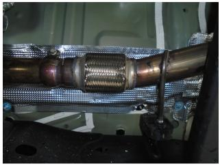
**Step 2.** To begin, fasten the Front Resonator Assembly to the outlet of the OE system using the OE clamp and by fitting the welded hanger into the rubber insulator (Leave all clamps and fasteners loose for final adjustment of the complete system.)
