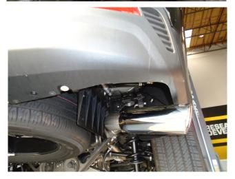
**Step 5.** Complete the installation by attaching the Tailpipe Assembly to the Pipe Assembly using the Supplied 3.00" clamp. Engage the welded hanger to the rubber insulator.
