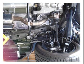
**Step 4.** Next loosely attach the Pipe Assembly to the Muffler Assembly using the supplied clamp. Engage the welded hanger to the rubber insulator.
